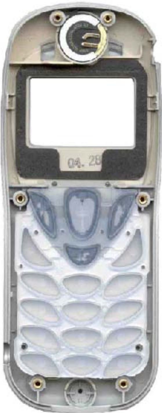
Front Housing (Internal View)
