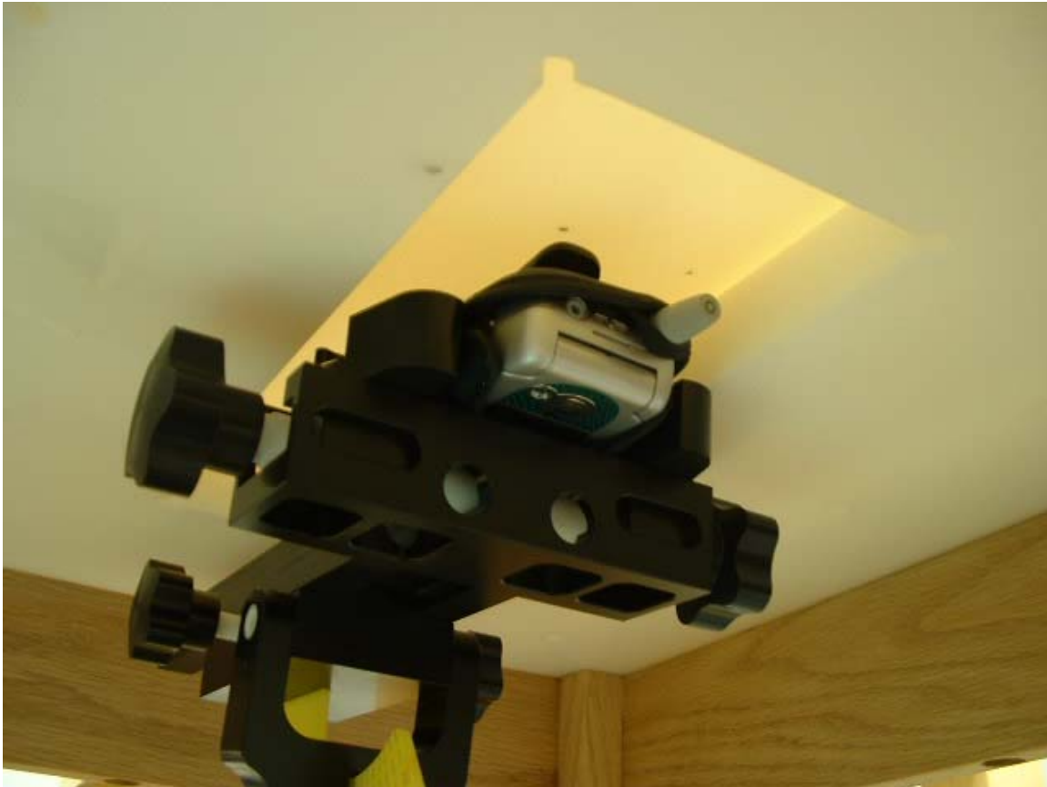
Figure 15. Phone with accessory pouch against the flat phantom (Body worn condition)
