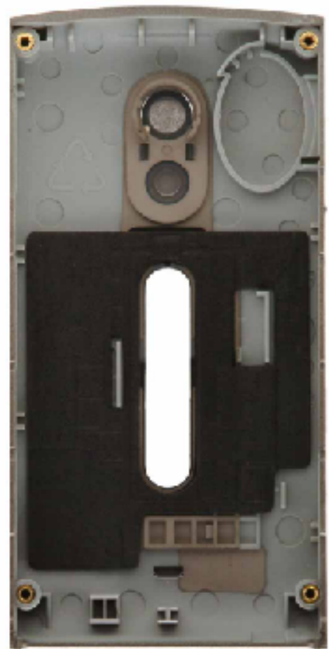
Upper Board Housing Internal View
