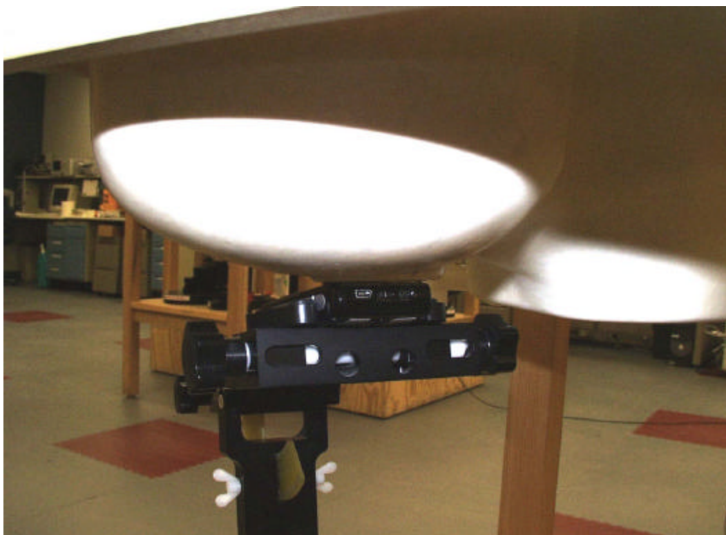
Figure 11. Phone Against the Head Phantom (Back View – 15° Tilt)
