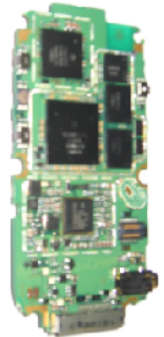
Main Board Front View (shields off)
