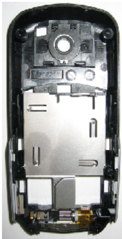
Rear Housing Internal View
