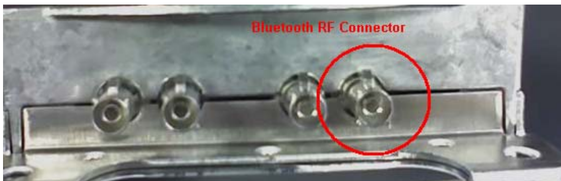
Figure 3: External side view showing the location of the Bluetooth RF connector. A Bluetooth antenna will be attached to the connector during the factory assembly process.
