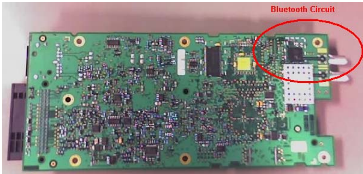
Figure 4: Internal front view with the Bluetooth circuit circled.
