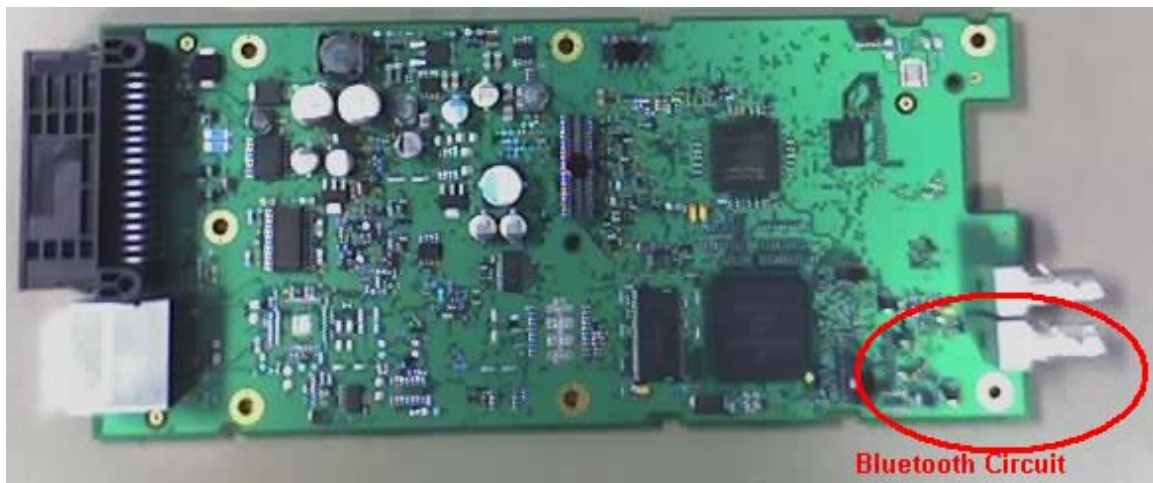
Figure 5: Internal rear view with the Bluetooth circuit circled.
