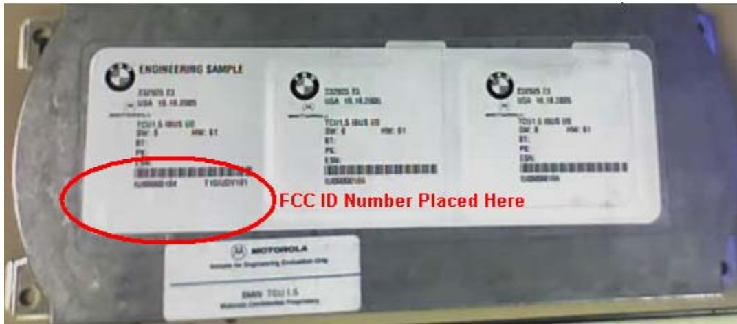
Figure 1: External front view. FCC label location circled.
