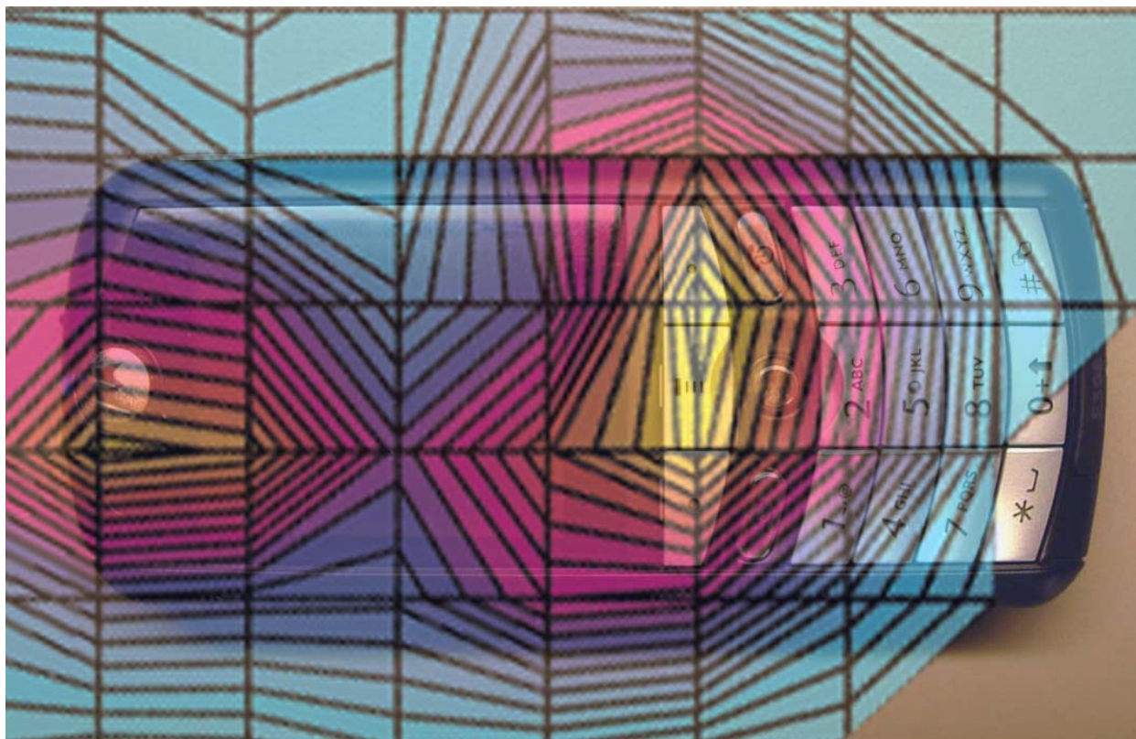
Figure 3. Typical 1900MHz Right Head Adjacent Contour Overlaid on Phone with Antenna Fixed (Cheek Touch)
