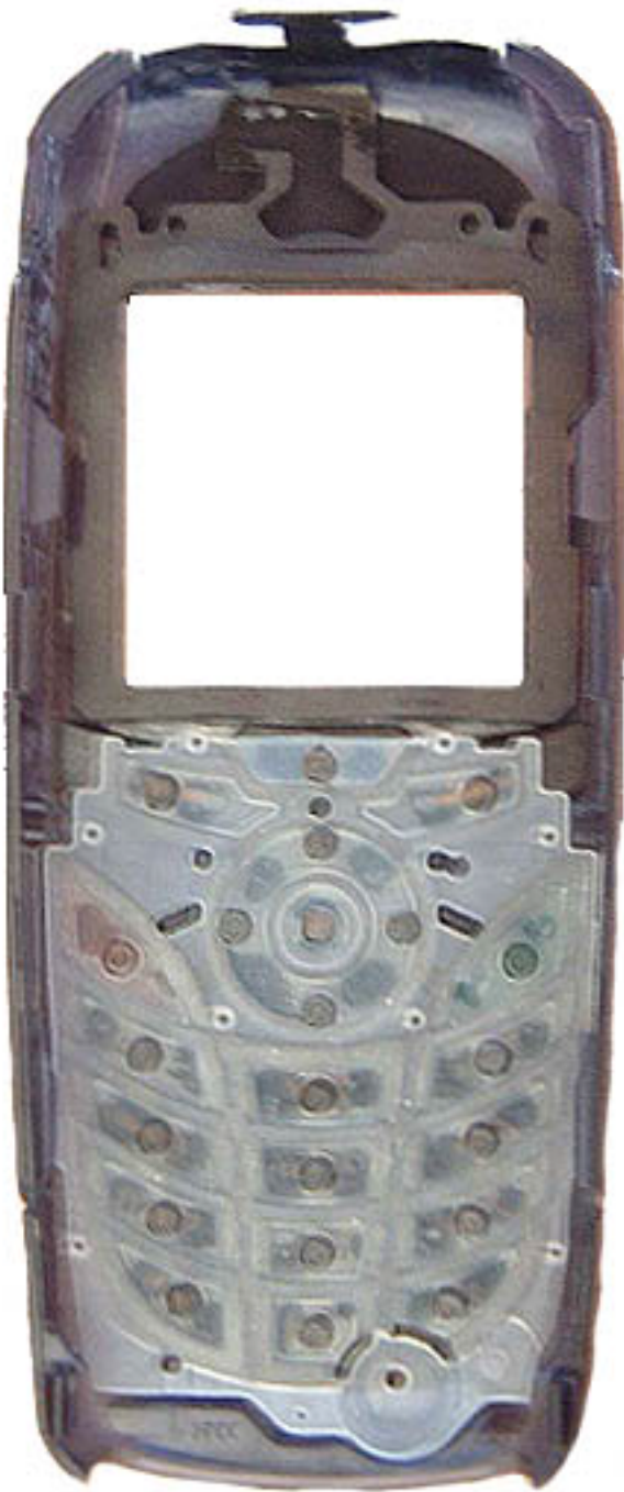
Front Housing Internal View
