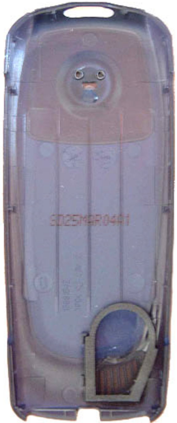
Rear Housing Internal View
