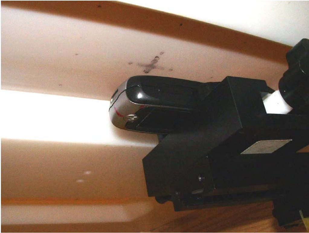
Figure 11. Body Worn Testing
