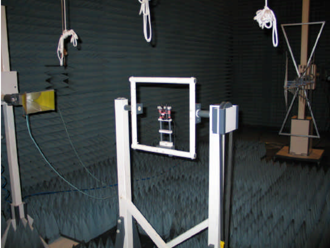
Photo 1: Test setup for radiated measurements
