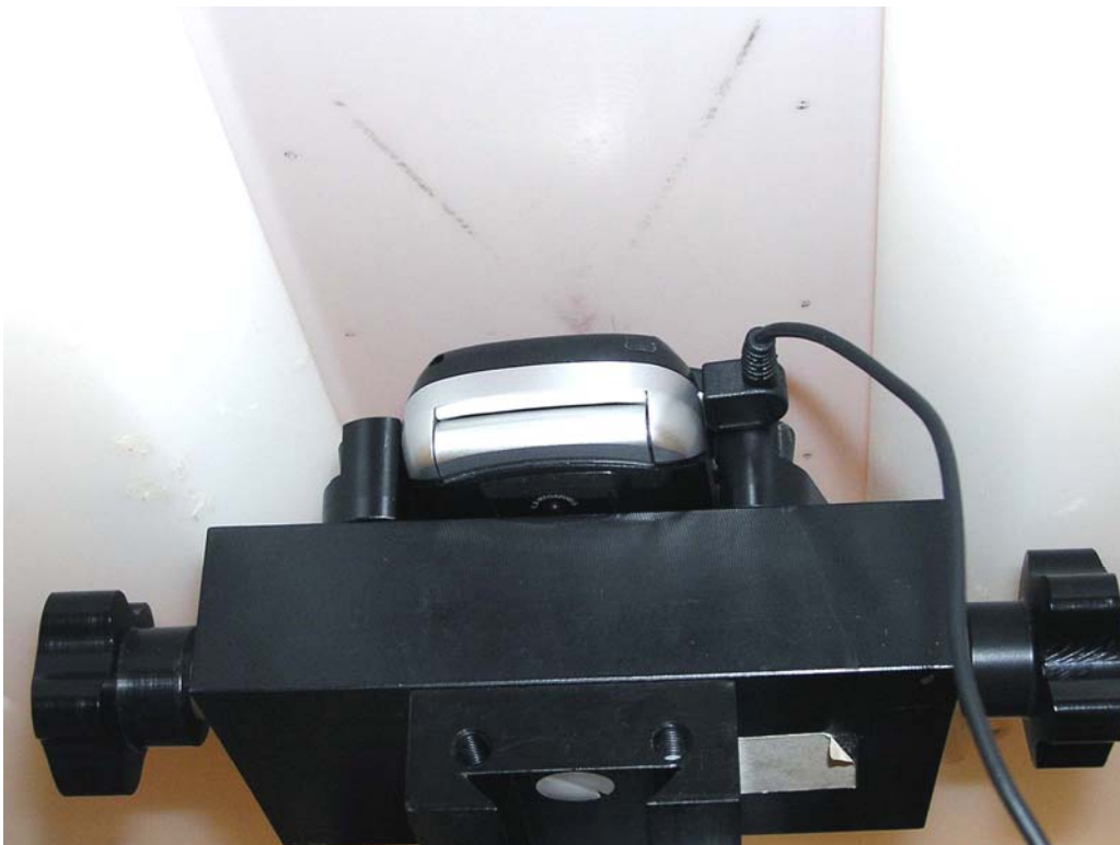
Figure 4. Phone Against the Flat Phantom
