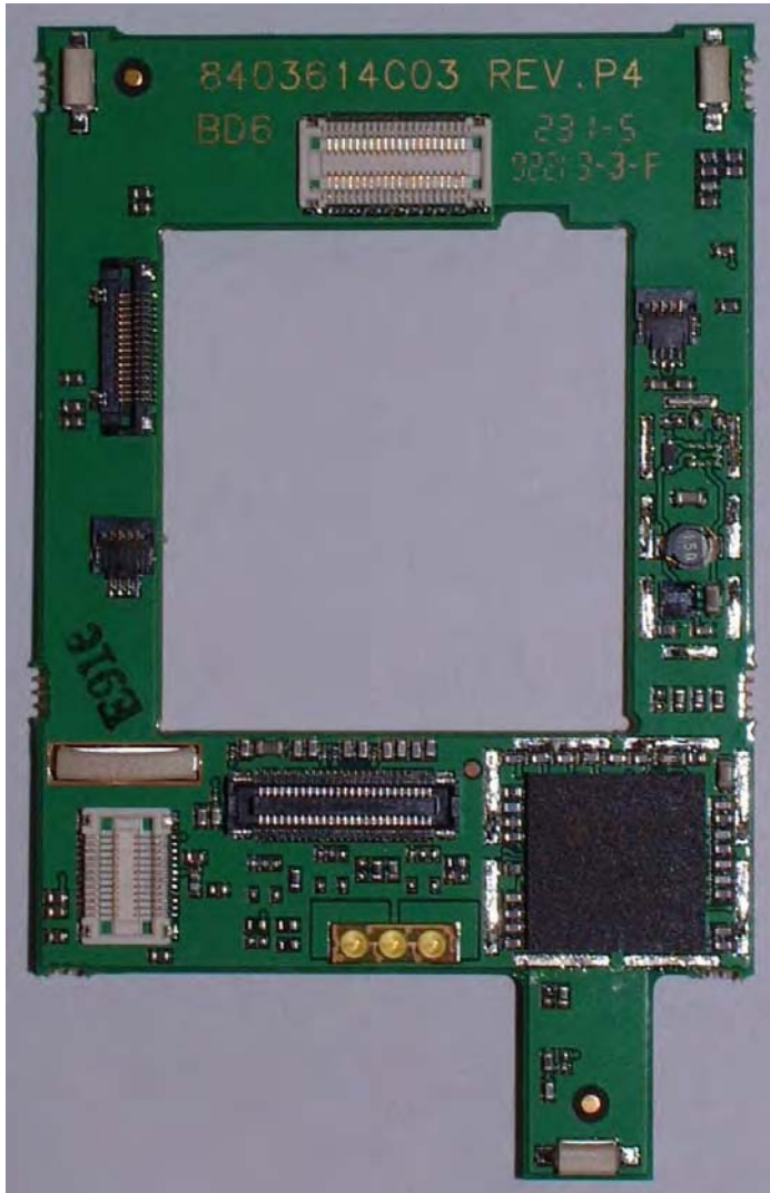
Flip Board without shields
