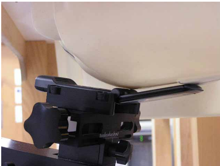
Figure 4. Phone Against the Head Phantom (Cheek Touch)
