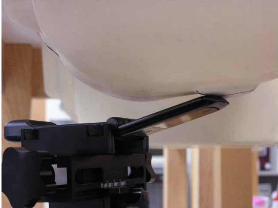
Figure 5. Phone Against the Head Phantom (15°Tilt)
