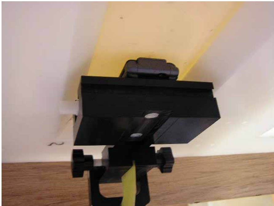
Figure 6. Phone Against the Flat Phantom
