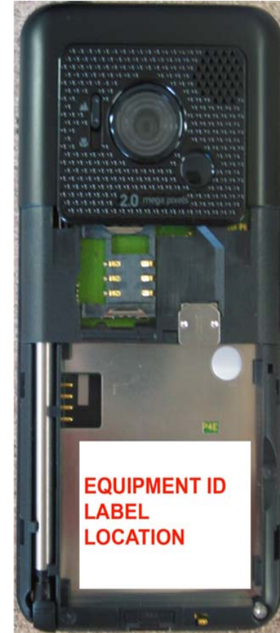
BACK OF PHONE WITH BATTERY COVER REMOVED
