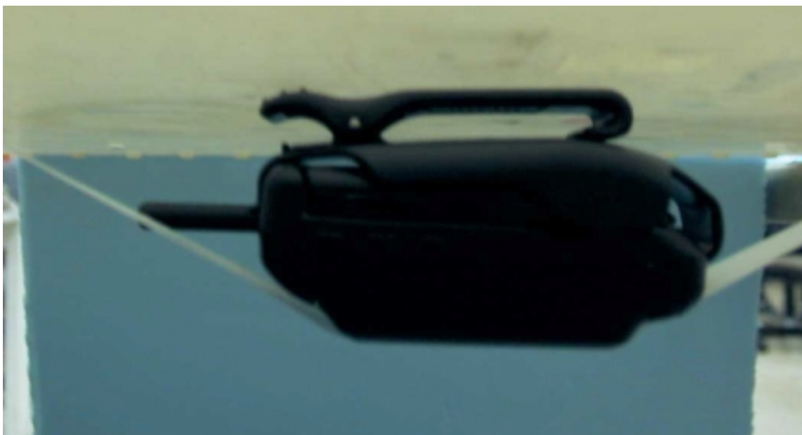
Figure 9. Phone In Supplied Belt Clip Against Phantom
