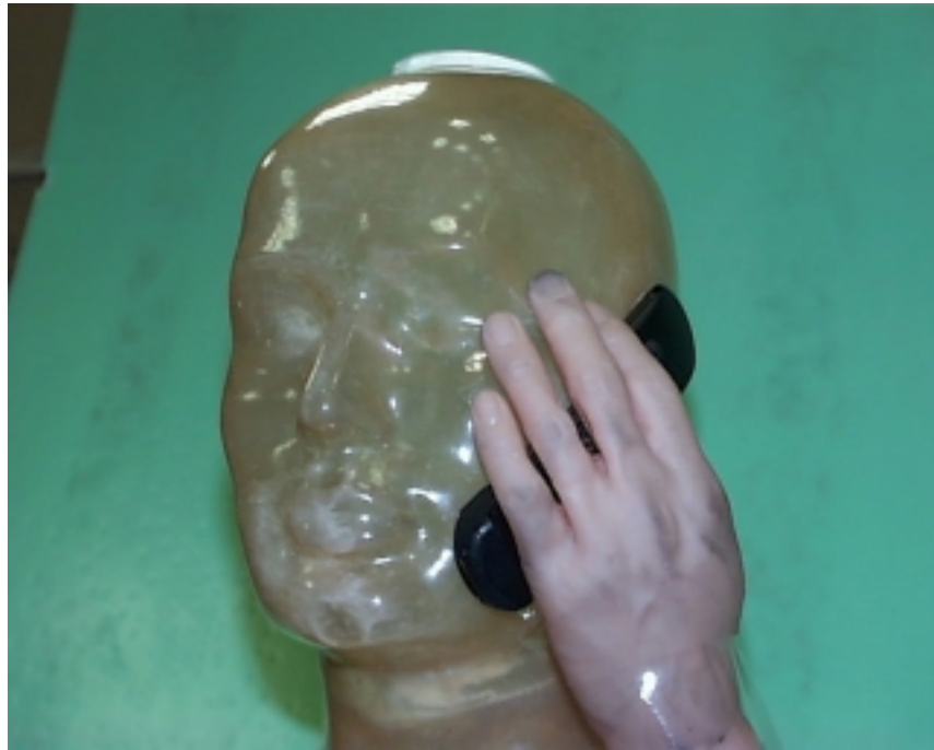
Figure 7. Simulated Hand Against Phantom Head.
