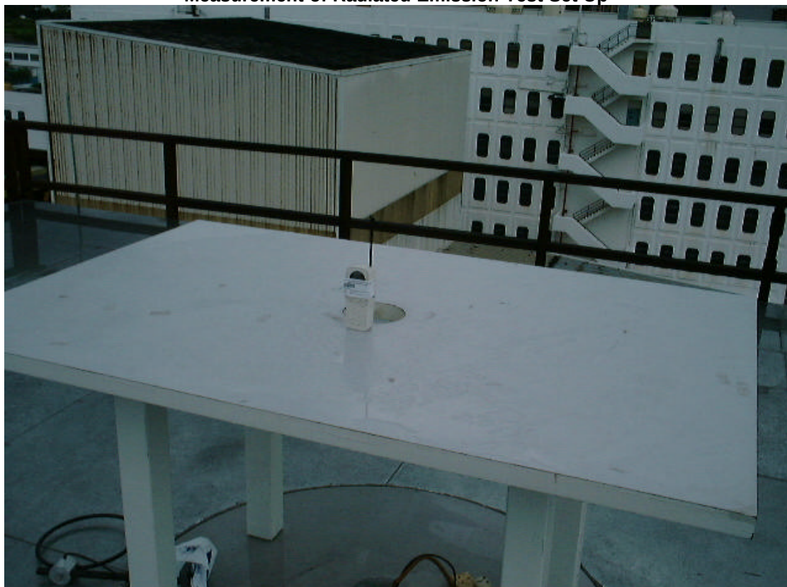
Measurement of Radiated Emission Test Set Up
