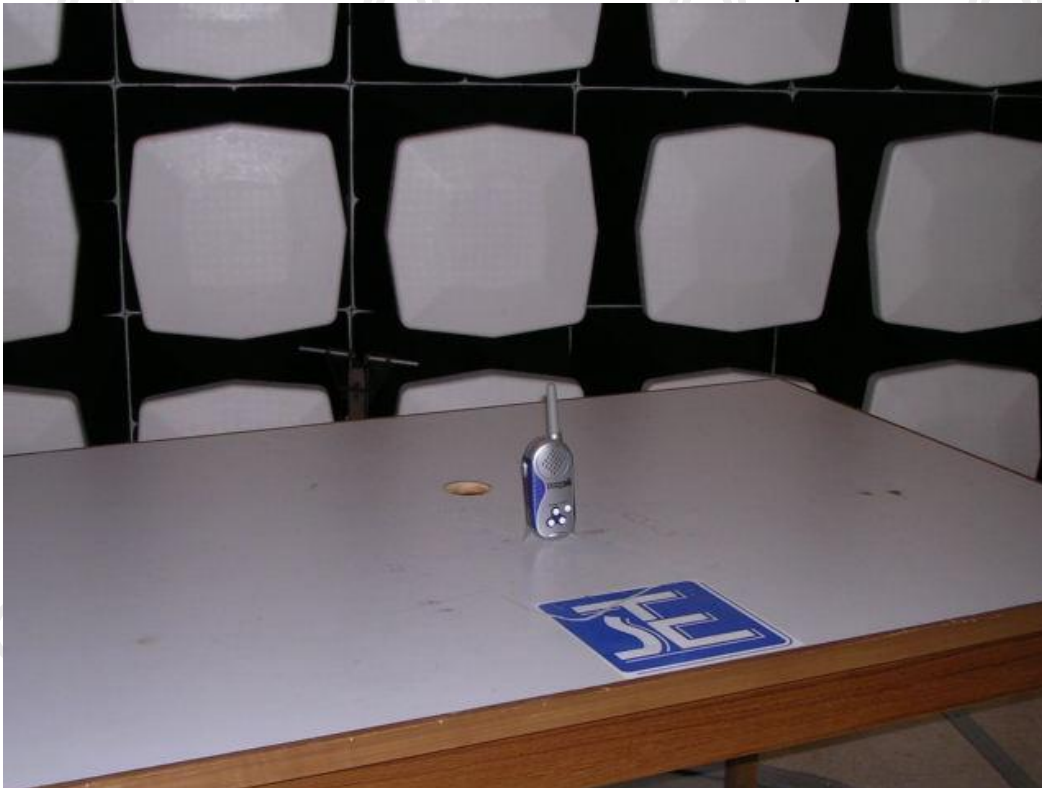
Measurement of Radiated Emission Test Set Up
