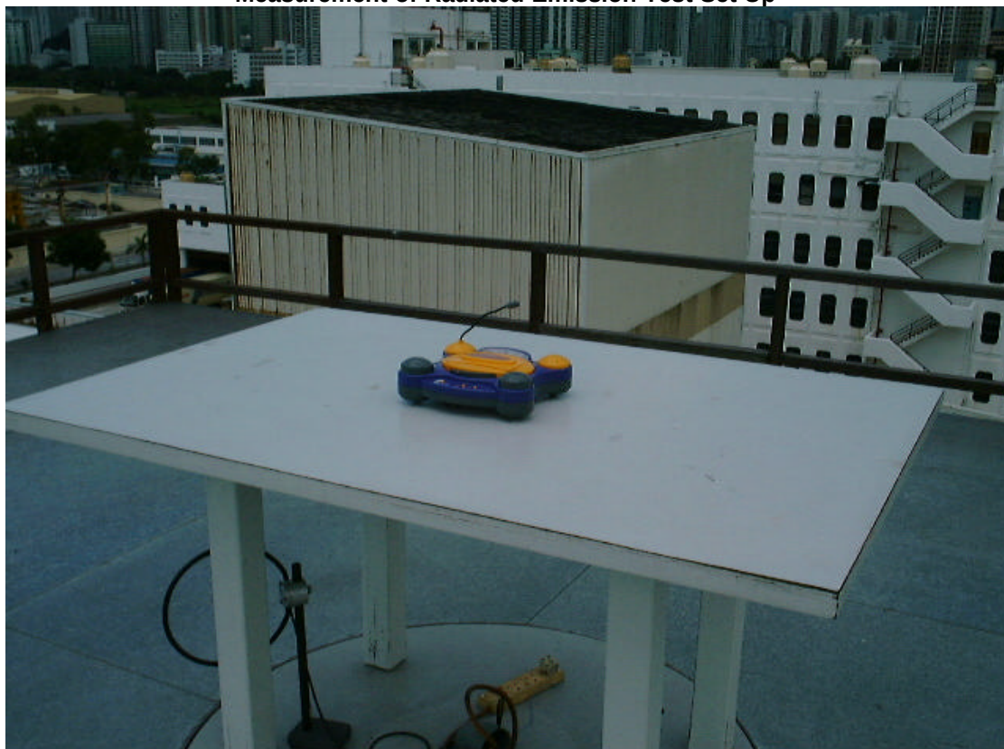
Measurement of Radiated Emission Test Set Up
