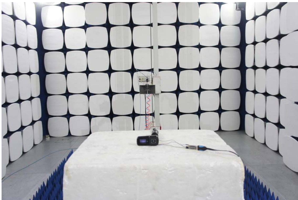
Radiated Setup photo (Above 1G)
