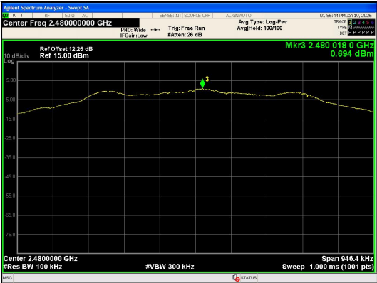
In-Band Reference Level BLE 1M_Channel 39
