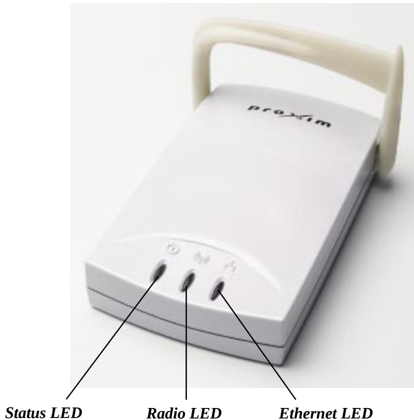
Figure 1 Harmony 802.11b Access Point's Top Panel LEDs
