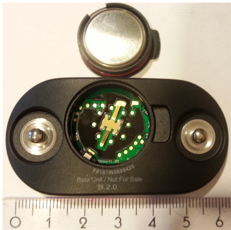
Figure 5. Battery cap opened.
