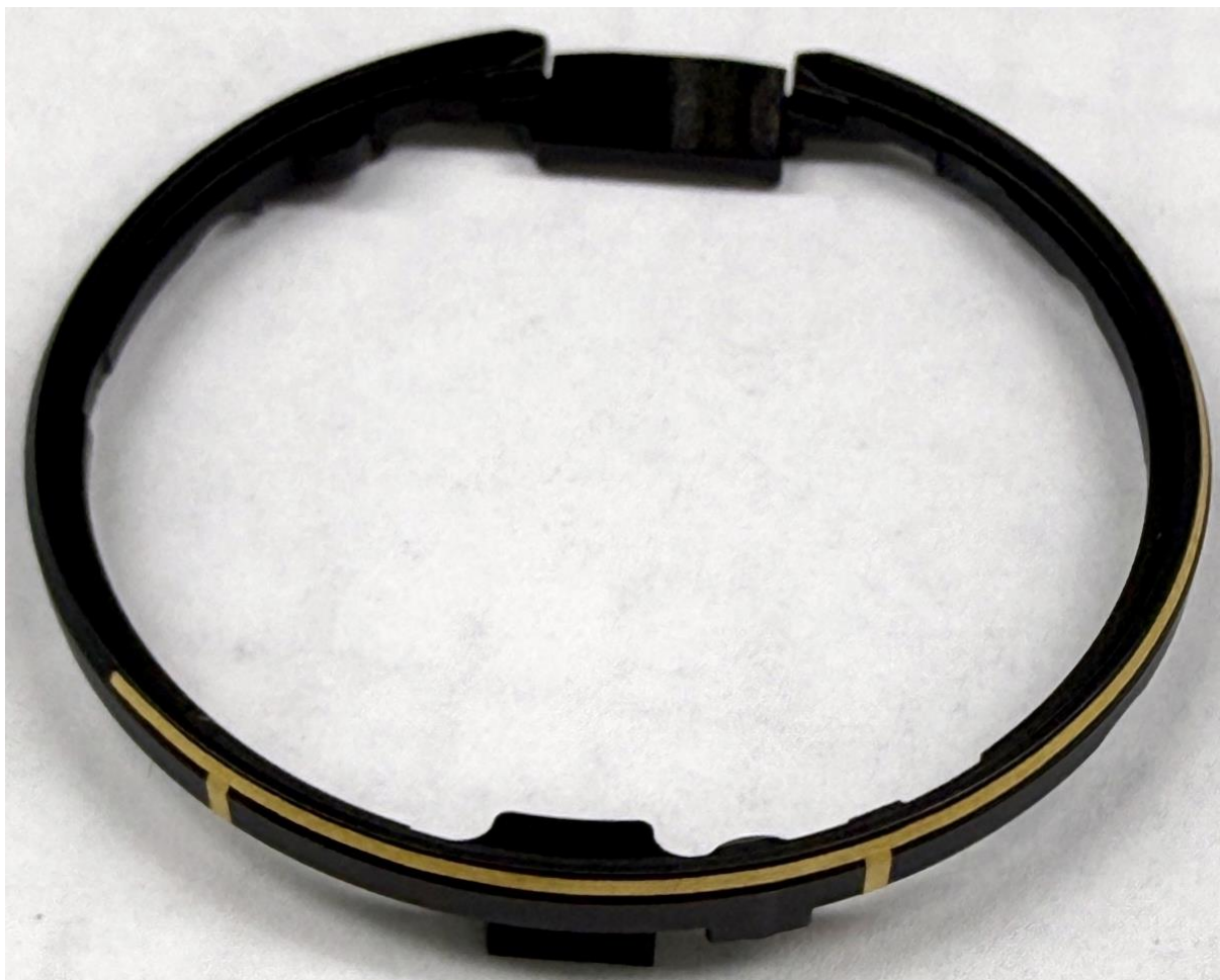
Figure 5. Antenna frame from the other side..
