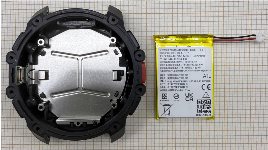
Figure 11. Battery removed, battery shield visible.
