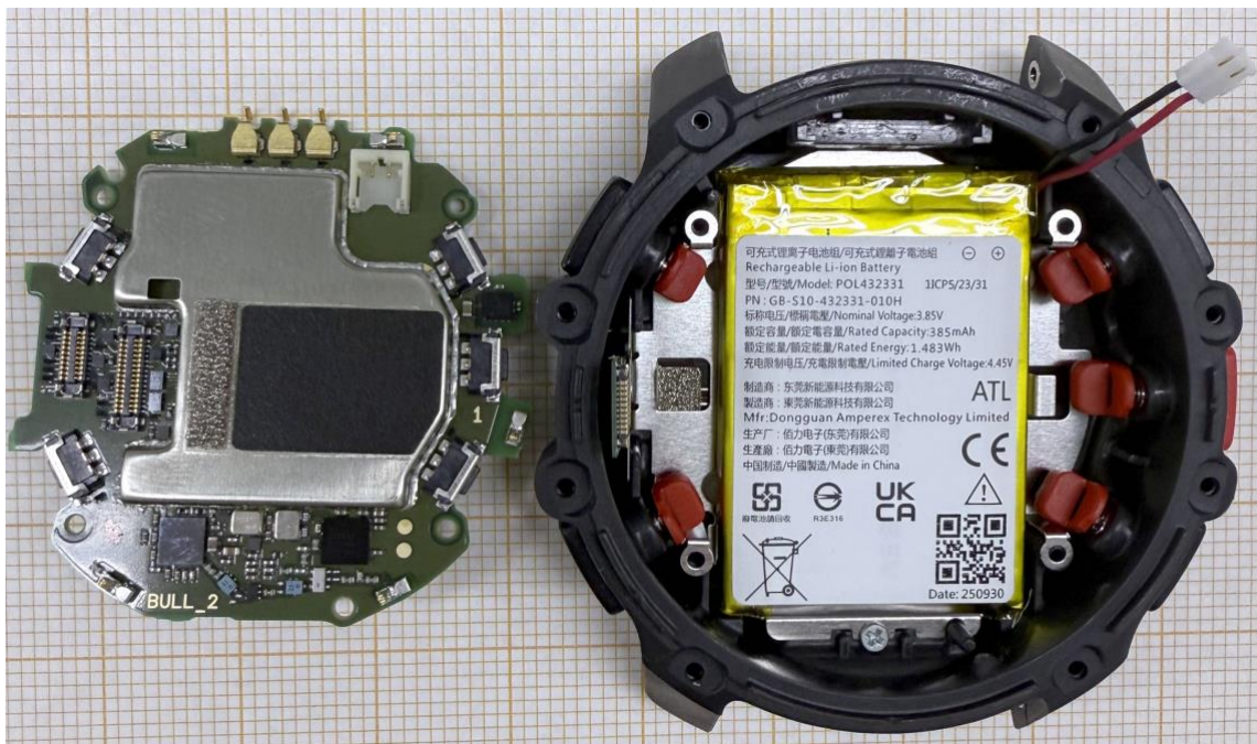
Figure 6. The main PWB removed, device battery visible.
