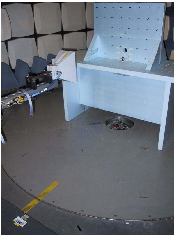
Picture 1: Spurious emission measurement setup
