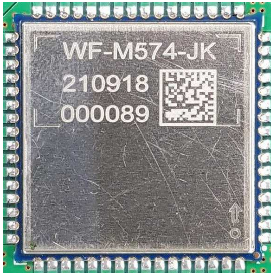
Radio Module (with Shielding case)
