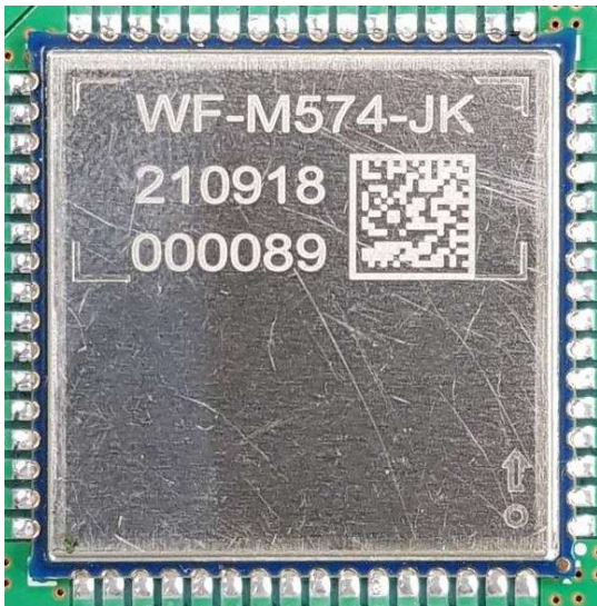
Radio Module (with Shielding case)
