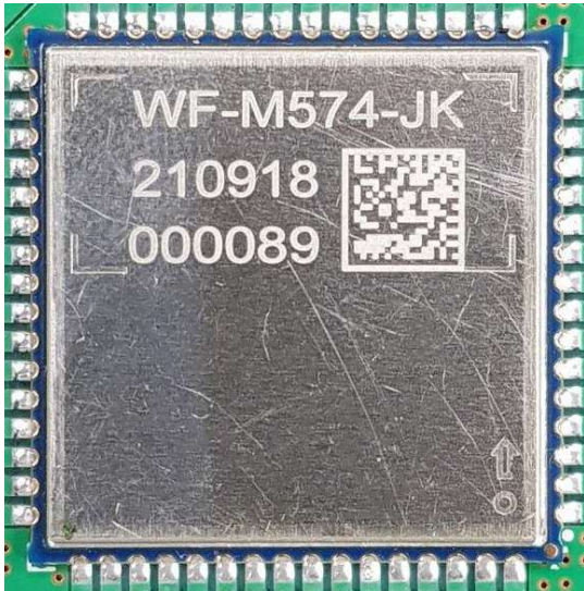
Radio Module (with Shielding case)
