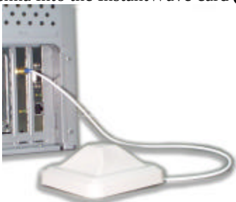
FIGURE 5. CONNECTING THE ADAPTER CARD ANTENNA
