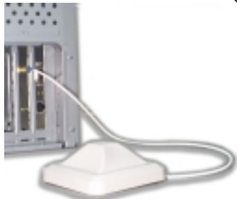
FIGURE 5. CONNECTING THE ADAPTER CARD ANTENNA
