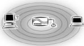
Figure 1. Simple Wireless Infrastructure Network
