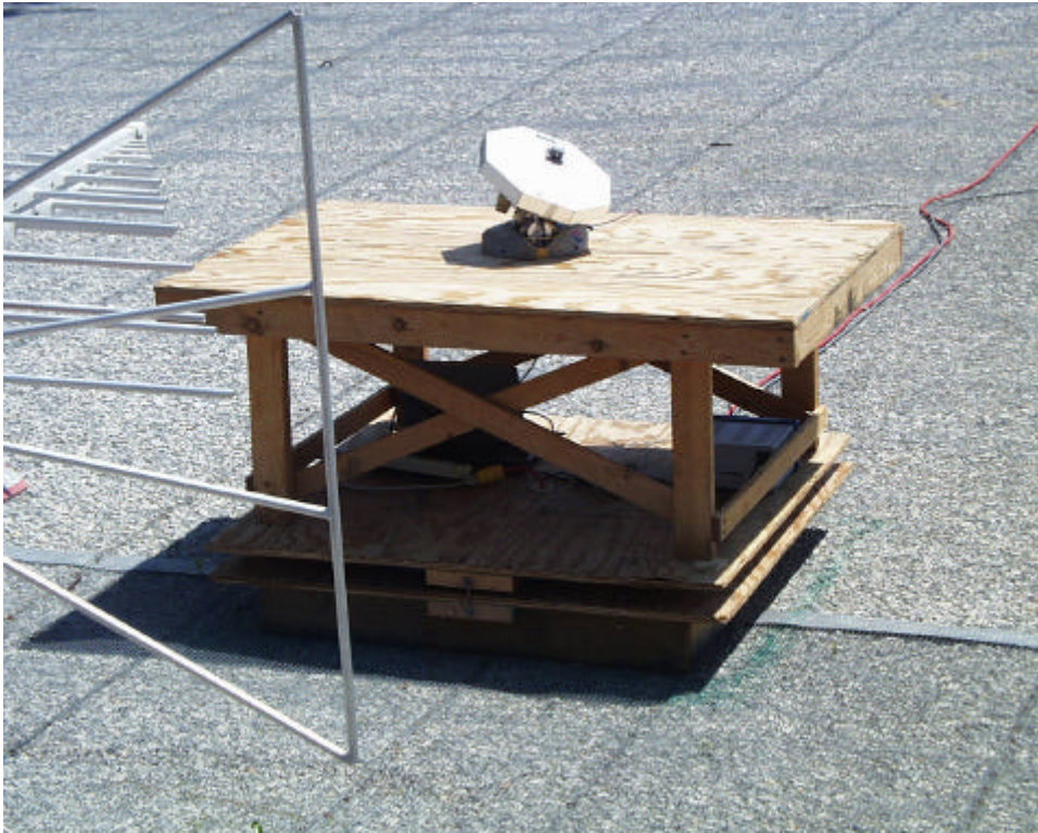
General emissions setup with load over antenna.
