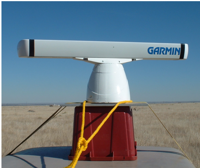
Figure 8. EUT mounted on the test platform.
