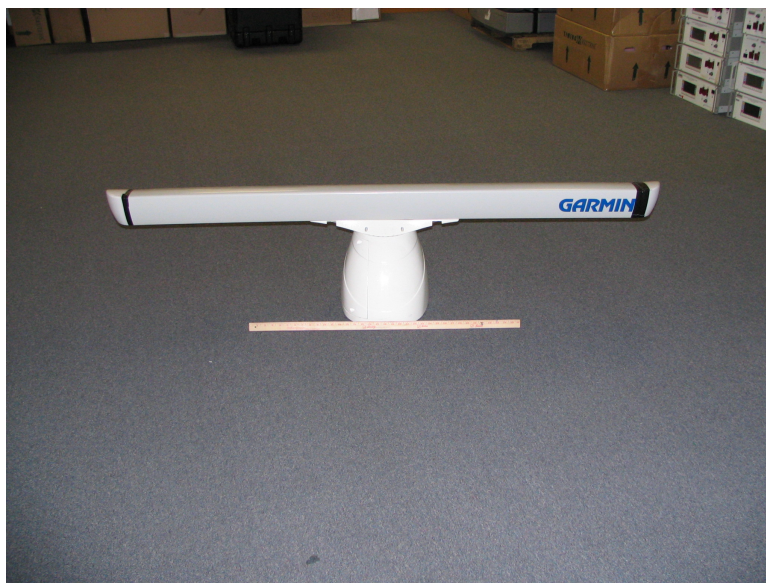
Figure 9. Interior of EUT. The radiating element is 180 cm between endpoints.
