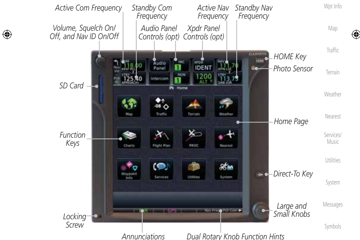
Figure 1-4 GTN 750 Front Panel
