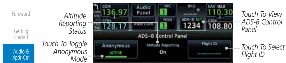
Figure 2-10 ADS-B Control Panel
