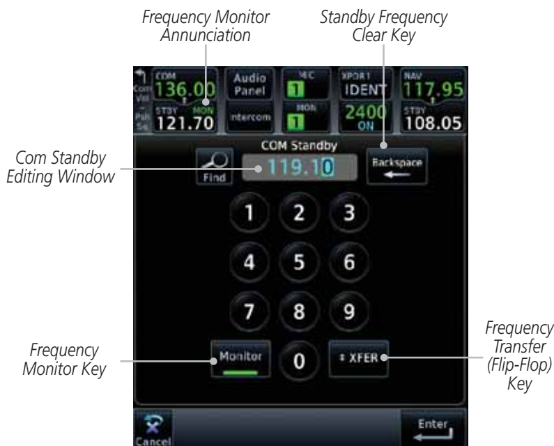
Figure 3-24 Com Frequency Monitoring
