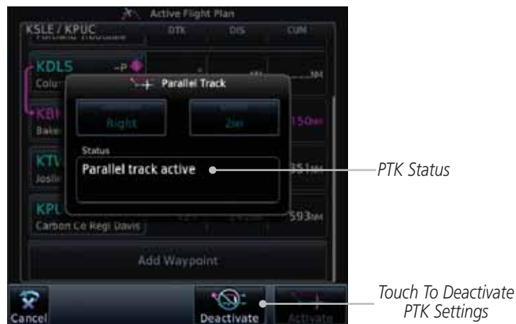
Figure 4-41 Deactivating Parallel Track
