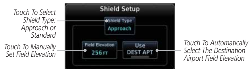
Figure 10-28 TCAD 9900B Shield Setup for Approach
