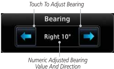
Figure 12-64 Bearing Line Adjustment
