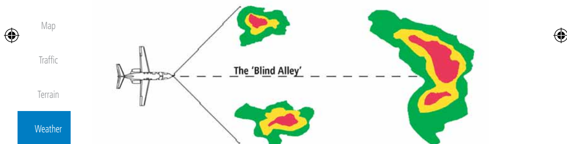
Figure 12-55 The “Blind Alley” Overhead View
