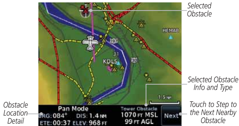
Figure 9-23 Point Obstacle Detail
