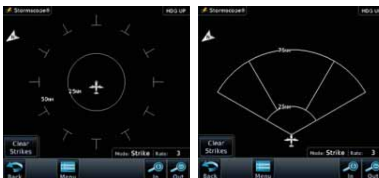
Figure 12-47 StormScope 360° and Arc Display Views
