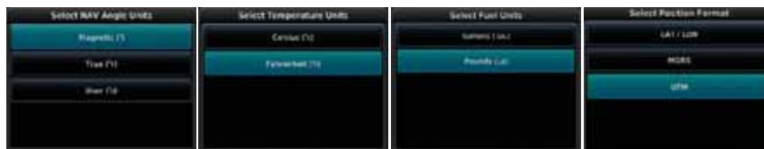
Figure 16-45 Setup Units Selection Windows
