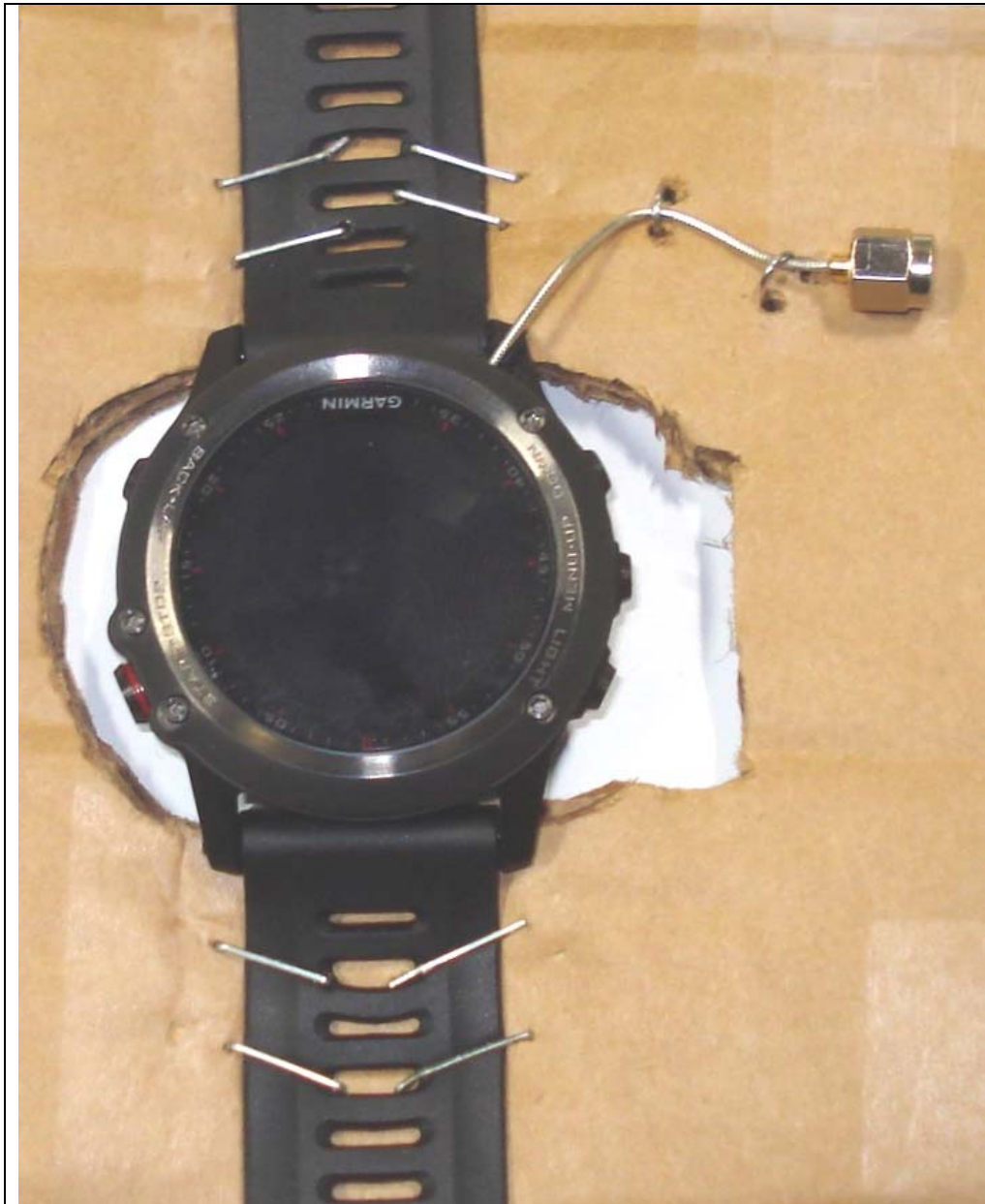
Modified for Conducted Power
