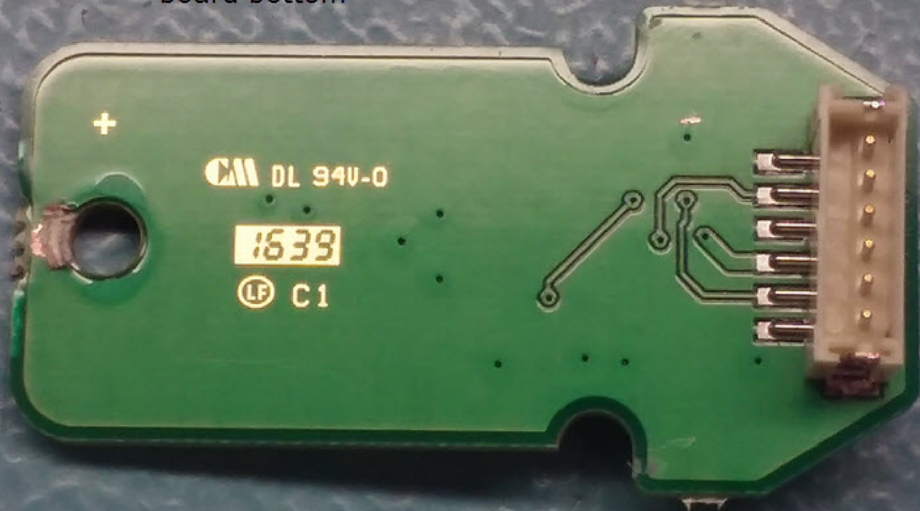
Antenna rotation sensor board bottom
