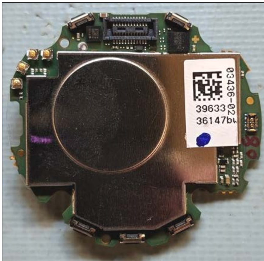
Main Board with Shield – Top View
