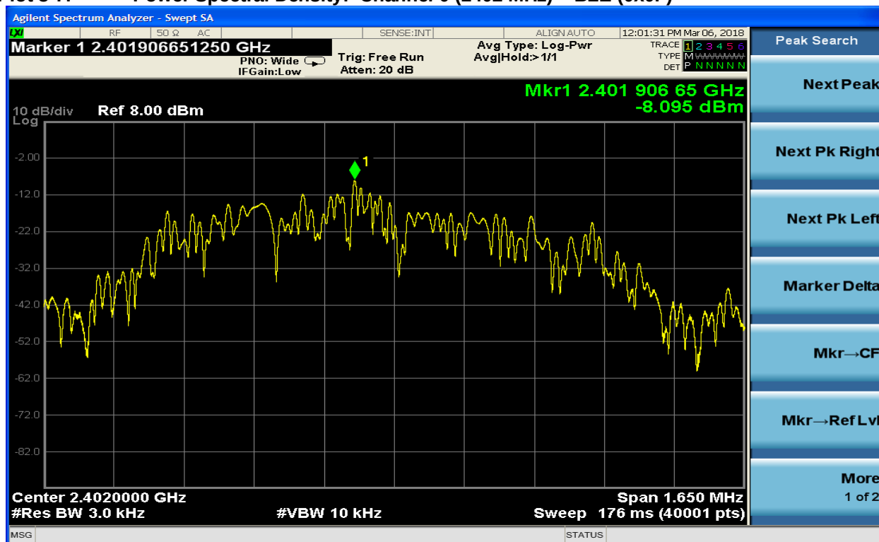
Plot 8-7: Power Spectral Density: Channel 0 (2402 MHz) – BLE (0x0F)
