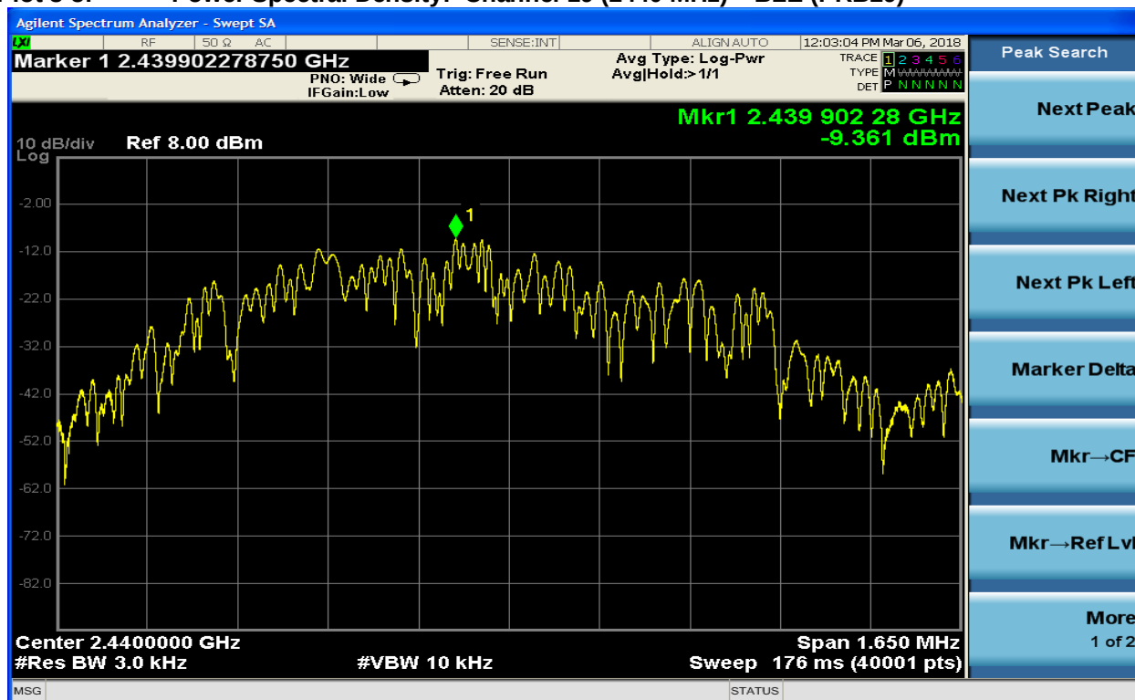
Plot 8-5: Power Spectral Density: Channel 19 (2440 MHz) – BLE (PRB29)
