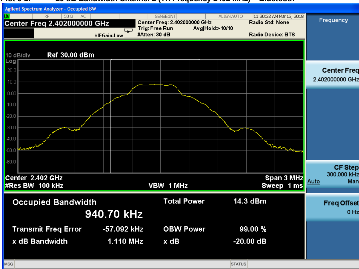
Plot 6-1: 20 dB Bandwidth Channel 2 (TX Frequency 2402 MHz) – Bluetooth
