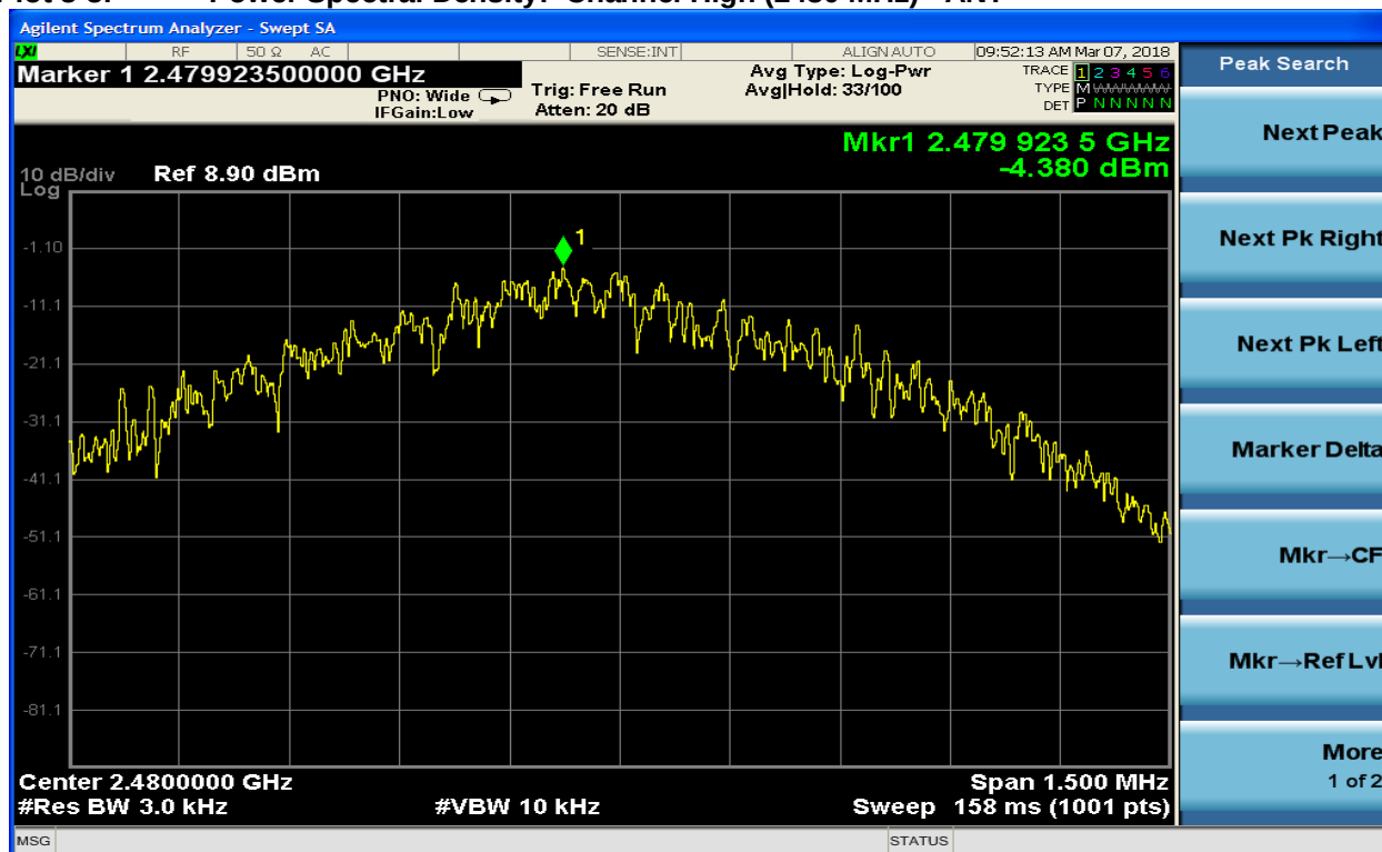
Plot 8-3: Power Spectral Density: Channel High (2480 MHz) - ANT+
