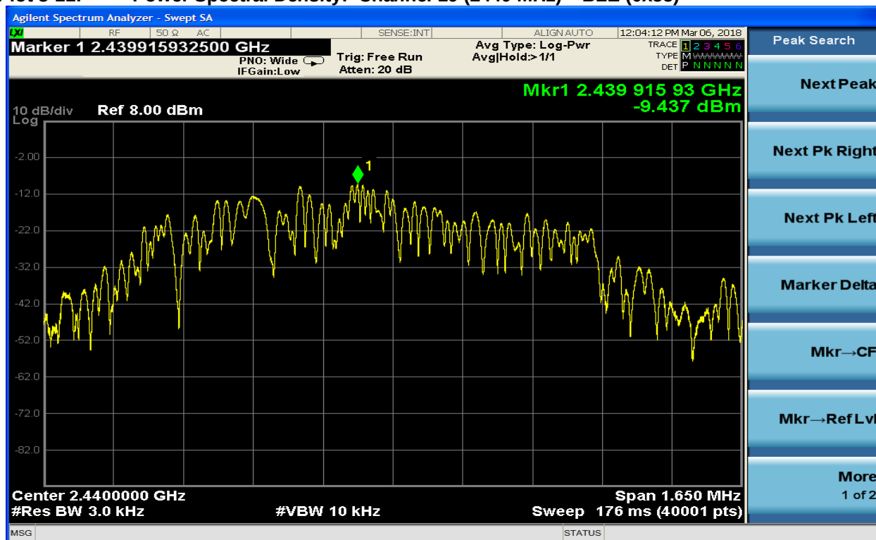
Plot 8-11: Power Spectral Density: Channel 19 (2440 MHz) – BLE (0x55)
