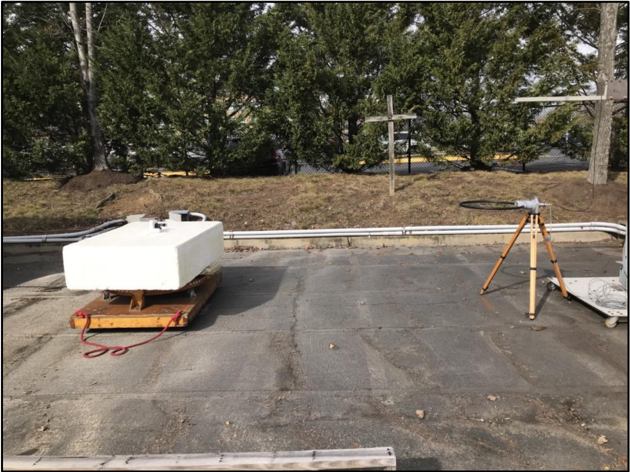
Photograph 2: Radiated Emissions Testing – Side View (Below 30 MHz)
