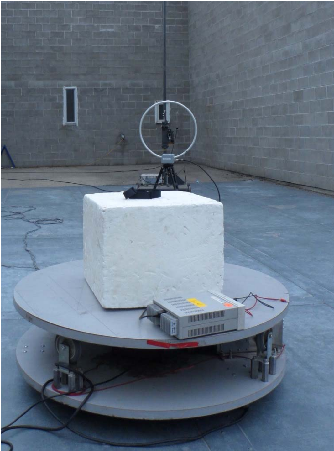
Figure E20.6 – Setup Photo – Radiated Measurements < 30MHz – Front
