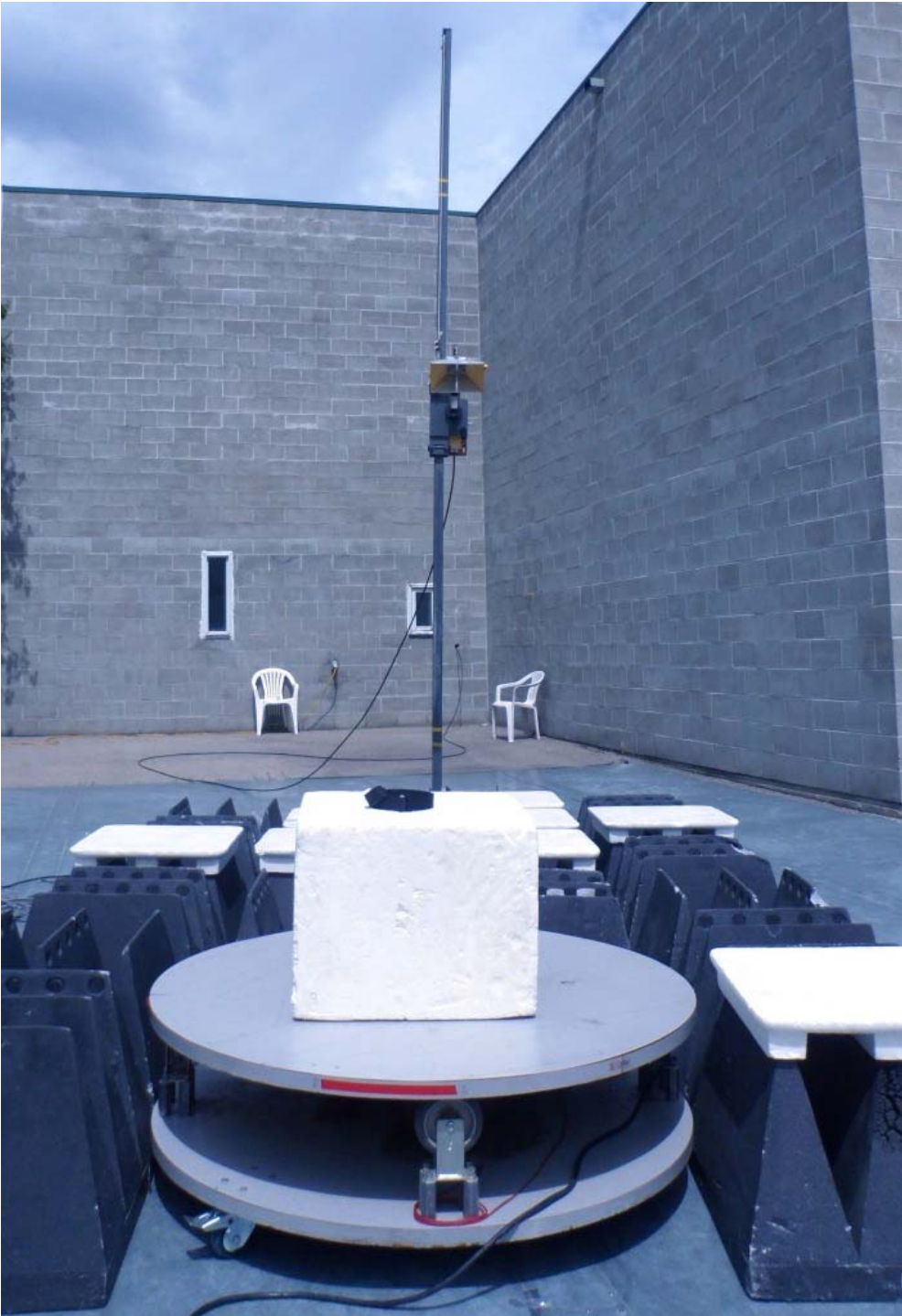
Figure E20.5 – Setup Photo – Radiated Measurements > 1GHz - Vertical
