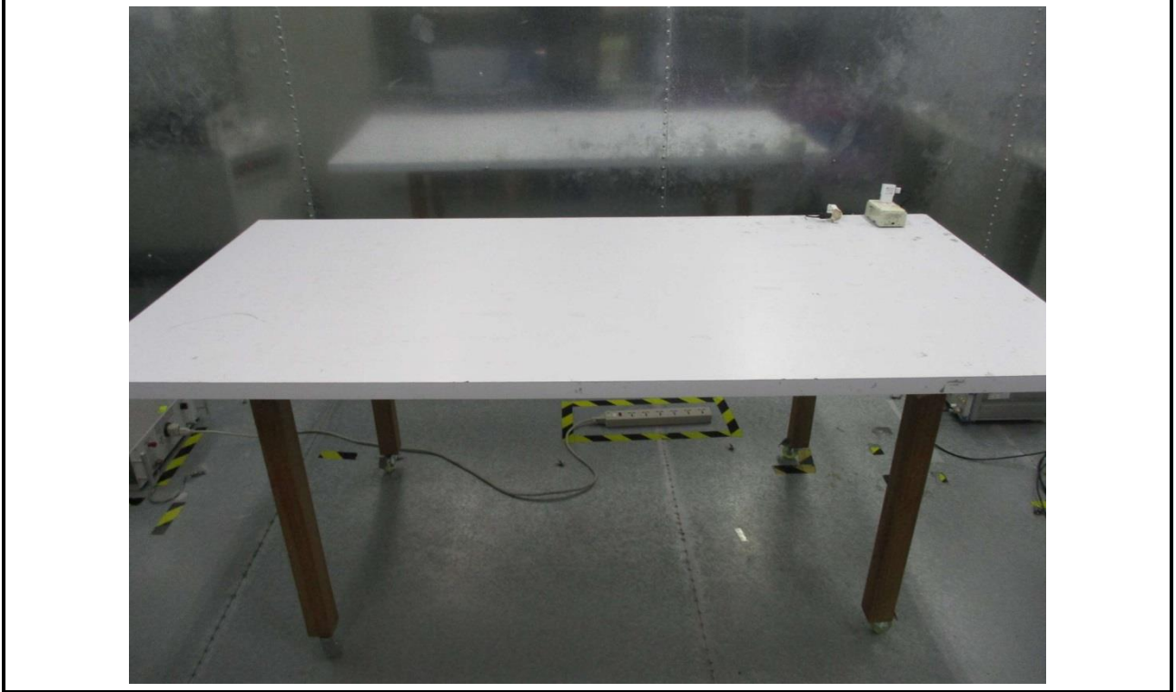
Conducted Emission Test (Charging mode)
