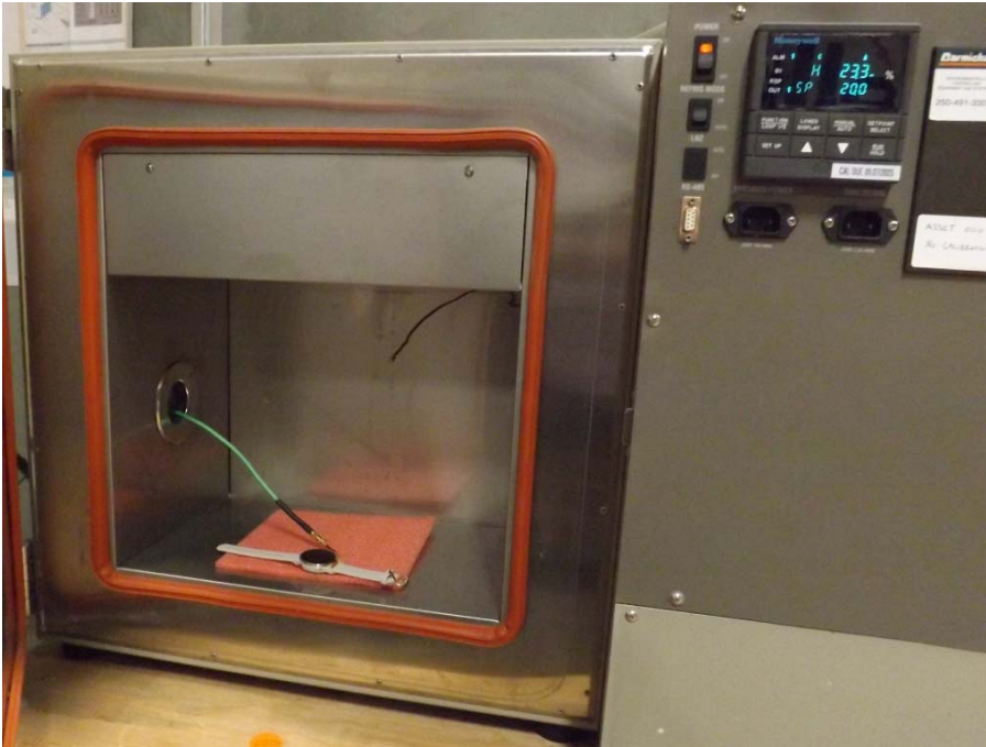
Figure E20.7 – Setup Photo – Frequency Stability
