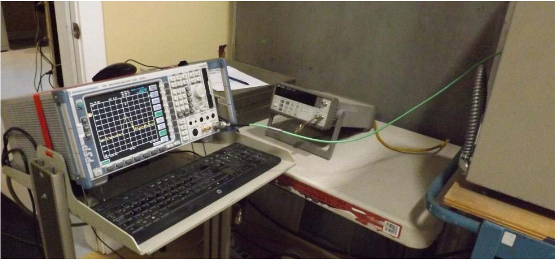
Figure E20.6 – Setup Photo – Frequency Stability
