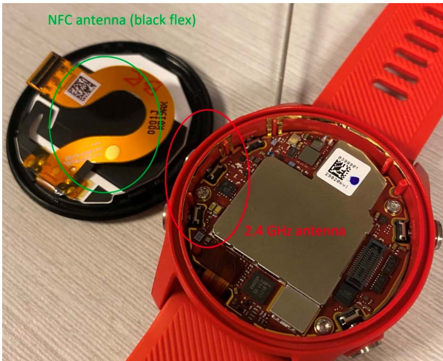
Figure E19.3 – Internal Photo – Antenna Locations
