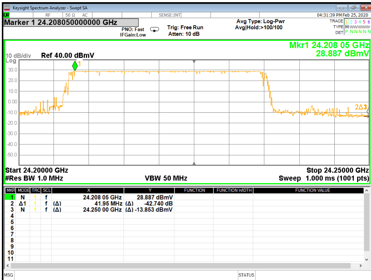
Figure 31 - Higher Band Edge (24 MHz) (swept frequency), 24.00 GHz Uncorrected measurement as recorded on spectrum analyzer, 5 cm test distance
