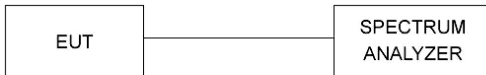
Figure 1 - Bandwidth Measurements Test Setup
