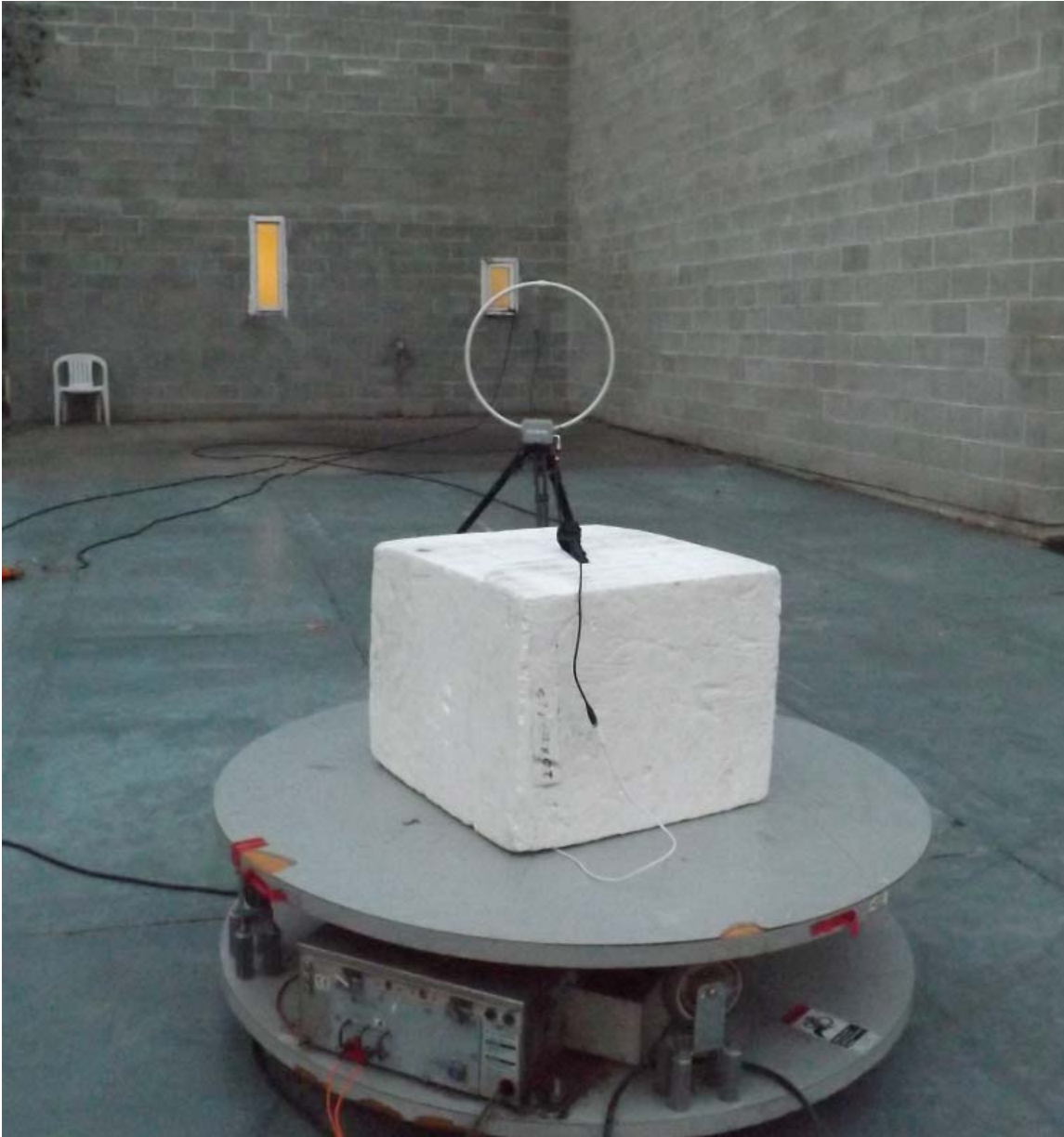
Figure E20.1 – Setup Photo – Radiated Measurements 9kHz – 30MHz
