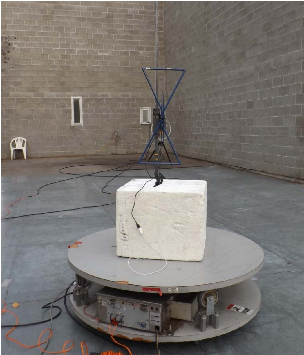
Figure E20.2 – Setup Photo – Radiated Measurements 30 - 1000MHz
