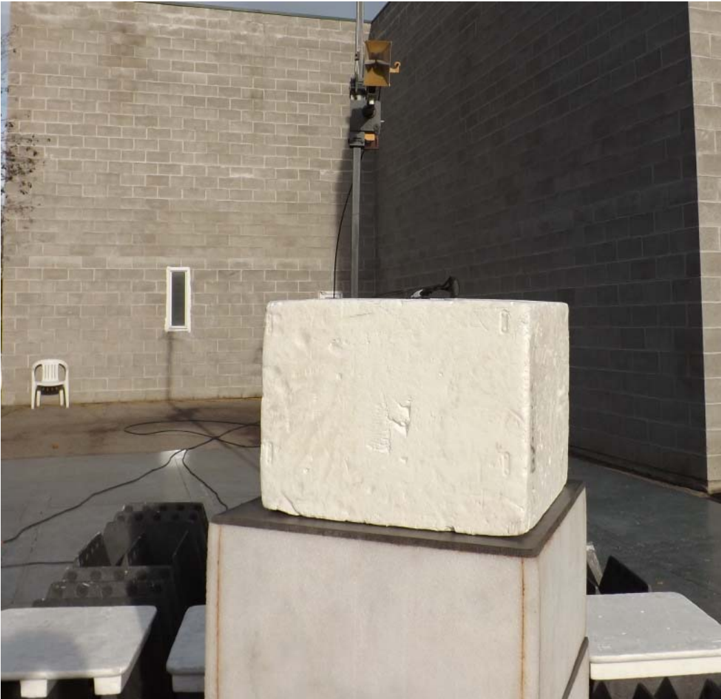
Figure E20.3 – Setup Photo – Radiated Measurements 1 – 18GHz
