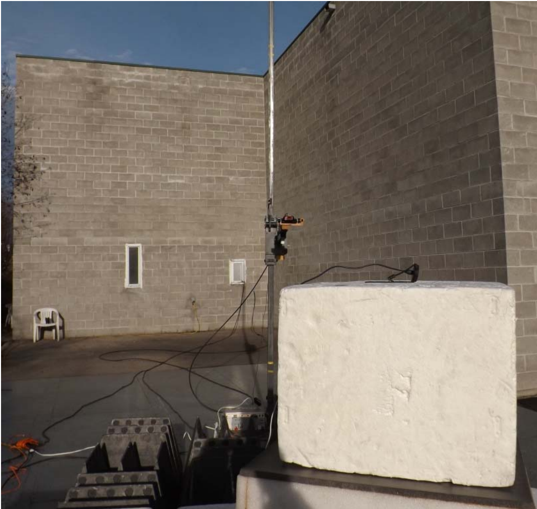
Figure E20.4 – Setup Photo – Radiated Measurements 18 – 26GHz
