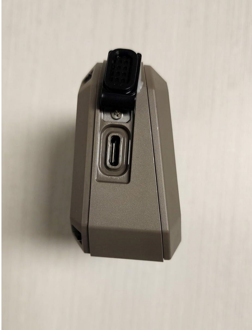
The right side of the EUT with USB-C slot
